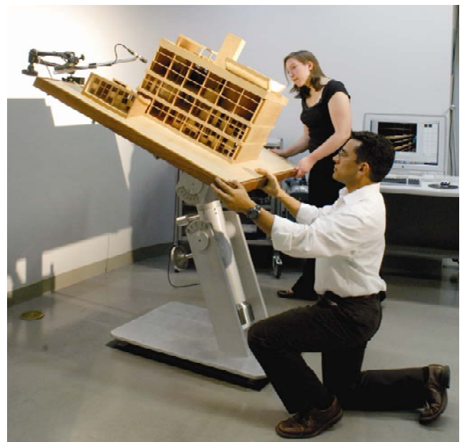
Staff of the Pacific Energy Center demonstrating the heliodon, a sun simulation device.
